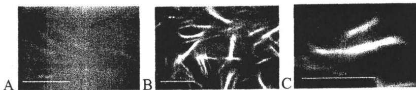
Figure 10. Fluorescence microscopy of [9]-12-[9]. A. Confocal image taken from wet gel. B. Taken after the gel was dried. C. One specific spot in the dried gel.
