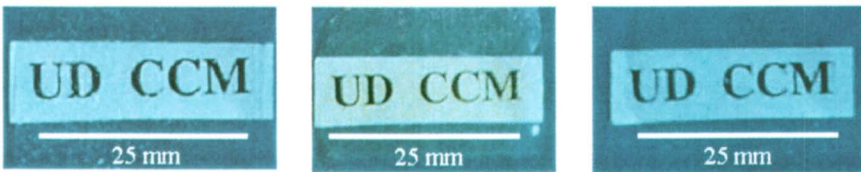
Plate 25.6. Nylon/Vinyl ester nanofiber composite films ~9 % fiber volume fraction
