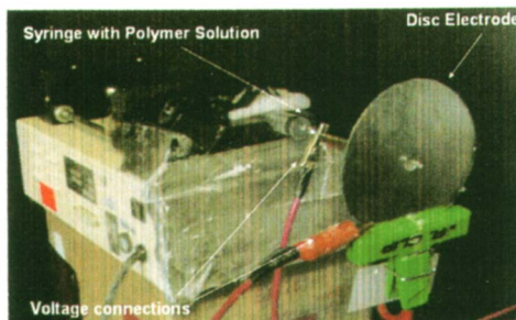
Plate 8.5. Electrospinning setup with the disc electrode (target not shown)
