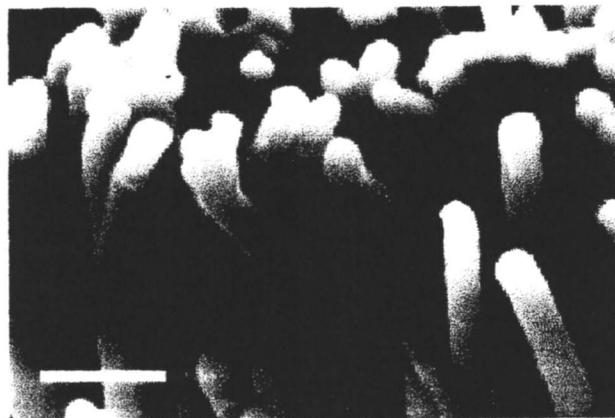
Figure 10. A typical SEM image of the CP-NT coaxial nanowires produced by cyclic voltammetry on the aligned carbon nanotube electrode, showing a thin layer of conducting polymer (polypyrrole) coating surrounding each of the constituent aligned carbon nanotubes. Scale bar is 1 \mu\text{m} . (Reproduced with permission from reference 37. Copyright 2000 Wiley-VCH Publishers, Inc.).
